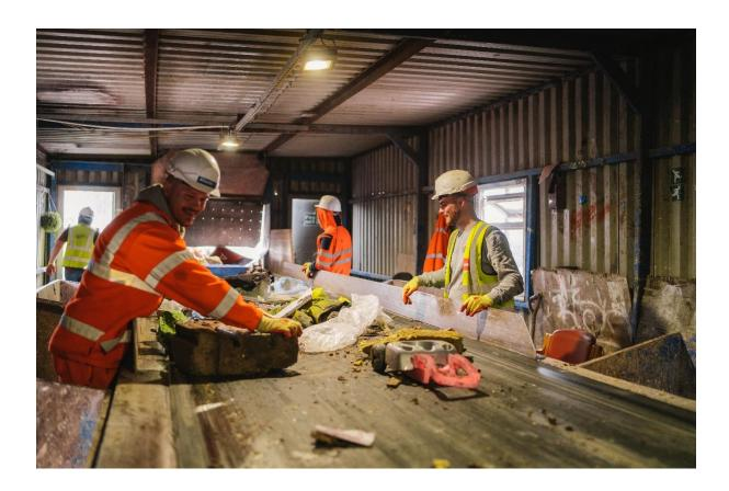
These materials are picked by hand from the conveyor belt and dropped via chutes into bays beneath the picking line from where the materials are collected and baled prior to storage for off-site recovery.
