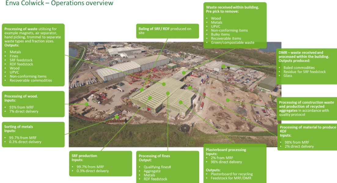
Figure 6.5 Enva Colwick layout and operations.
